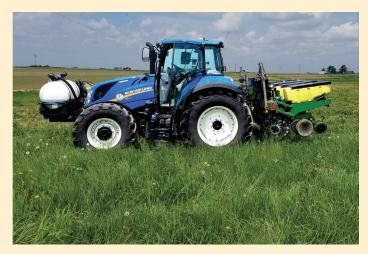
Research planter equipped with hydraulic row-unit downforce, various closing-wheel systems, and variable-rate starter fertilizer. Utilizing these technologies, planting corn in no-till production systems can help with emergence depending on soil conditions. Photo by Brian Luck.
